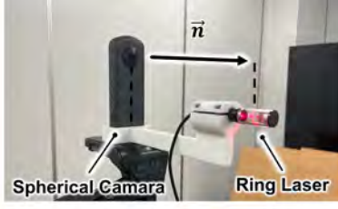
Fig.1 Developed sensor and relationship and camera and laser
