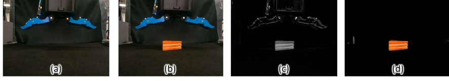
Fig. 2. Example of object detection: (a) Background image, (b) Foreground image, (c) Difference image between (a) and (b), and (d) Extracted object.
