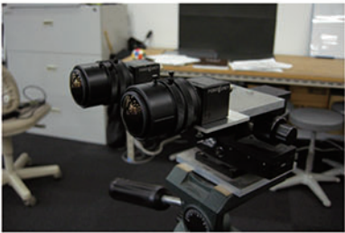
Fig.7 Fisheye stereo camera.
