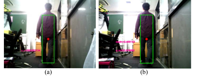
Fig. 5. Examples of points used for distance calculation: (a) left camera image and (b) right camera image.
