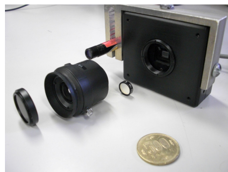
Fig.2 Decomposed status. From left, R72 filter, camera lens, band-pass filter, CCD camera.
