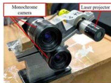
Fig.1 Appearance of sensor
