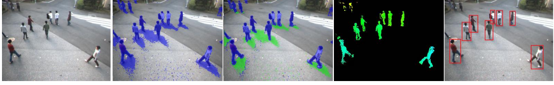
FIGURE 1. Overview of the proposed human detection algorithm based on subtraction stereo. Distance information of foreground regions are obtained from the subtraction stereo through shadow removal (green pixel in the center image). From left to right. Input image, foreground candidate obtained by subtraction stereo, shadow detection, disparity image, detected humans.
