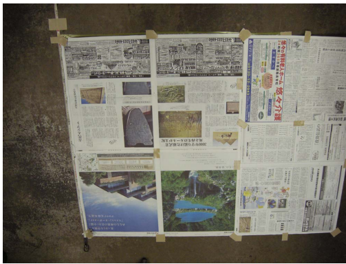
Fig. 13. measured object for the 3D mapping: the floor surface textured by a newspaper
