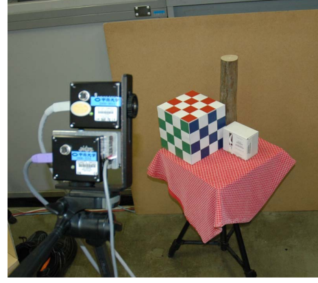
Fig. 11. Measured objects with the constructed sensor: from left, a cube with texture, a tree trunk, and a box of white cardboard
