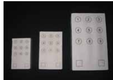
Fig. 5 Objects used for the button-pushing task: 83 \times 50 \times 17 [mm] (left), 100 \times 60 \times 20 [mm] (middle), 150 \times 90 \times 30 [mm] (right)
