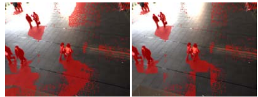
Fig. 1 Example of noise remove. On the left changes detected using the dinamic threshold. On the right remove of the noise
