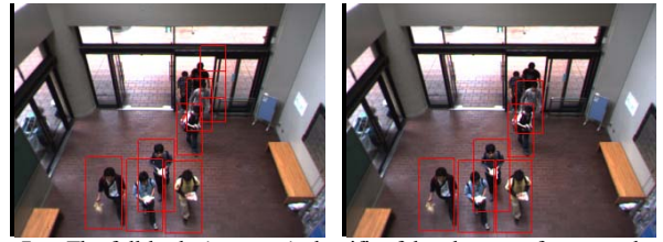
Fig. 7. The full-body (one-step) classifier false-detects a foreground region with the feature in the straight line direction of an intensity gradient like the automatic door (left). The hull-body (two-step) classifier is not detection the automatic door (right).
