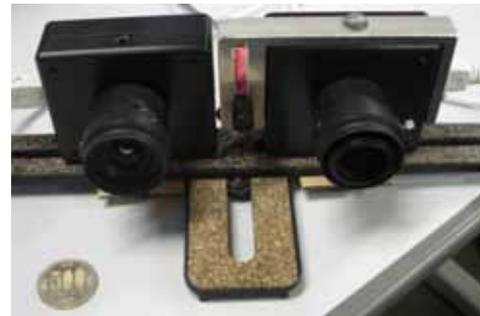
Fig. 1 Constructed sensor. From left, color CCD camera, laser projector and monochrome CCD camera with optical filter.
