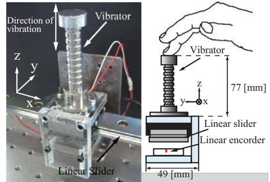
Fig. 6. Linear-slider-type interface
