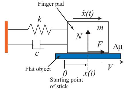
Fig. 2. 1-DOF vibration model of stick-slip motion
