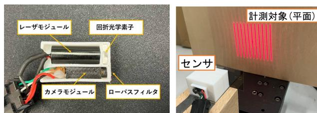
(a) Inside view of the sensor (b) Experimental environment
