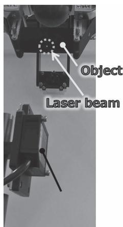
**Fig. 9** The setup used for data collection to evaluate metrics. The laser displacement sensor measures the position of a grasped object from below
