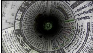
Fig. 9 Internal image of a transparent tube wrapped with newspaper.
