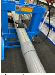
Fig.3: Deformation process of a pipe.
