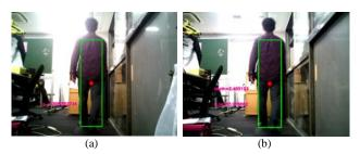
Fig. 5. Examples of points used for distance calculation: (a) left camera image and (b) right camera image.
