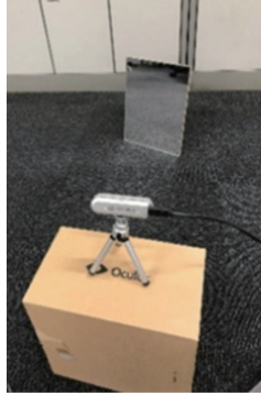
Fig. 3. Measurement scene with a mirror. Fig. 4. Acquired range image for Fig. 3.
