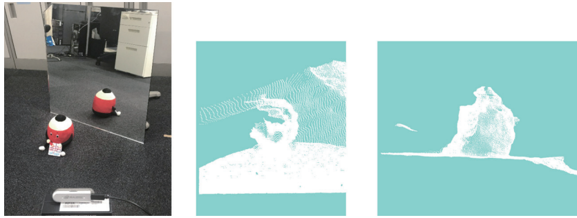
Fig. 7. An example of shape reconstruction: a stuffed toy. Left: measurement scene, center: top view, right: right-side view
