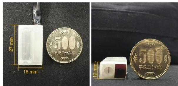
Fig. 1 Constructed range image sensor
