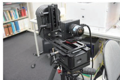
(a) Fisheye camera mounted on a rotation table
