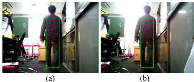
Fig.4 Examples of points used for distance calculation: (a) Left camera image and (b) Right camera image
