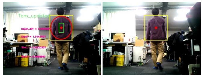
(a) Left camera (b) Right camera Fig. 4 Template matching between two cameras
