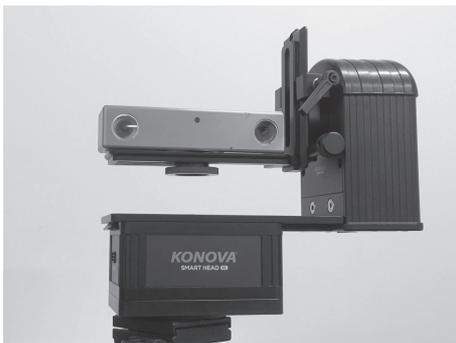
Fig. 7 Stereo camera mounted on a pan-tilt head.
