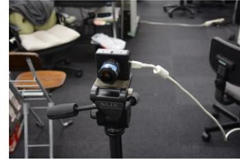
Fig. 11. Fisheye camera mounted on a tripod
