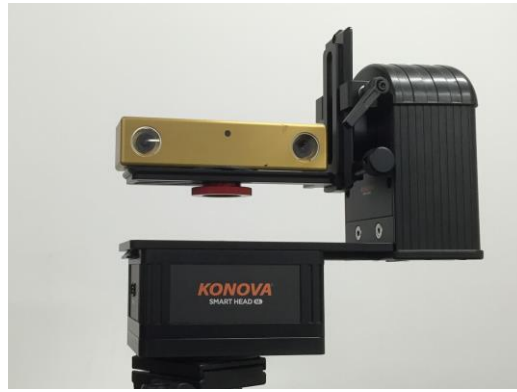
Figure 7: Stereo camera mounted on pan-tilt head
