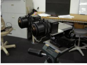
Fig. 6. The appearance of the fisheye stereo camera
