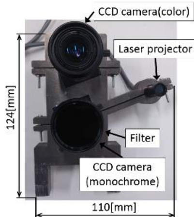
Fig. 1 Constructed compact range image sensor
