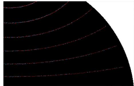
Fig. 5 Estimation result when maximum added error is 0.5 [pixel]. Blue dots are projected points and red dots are re-projected points.
