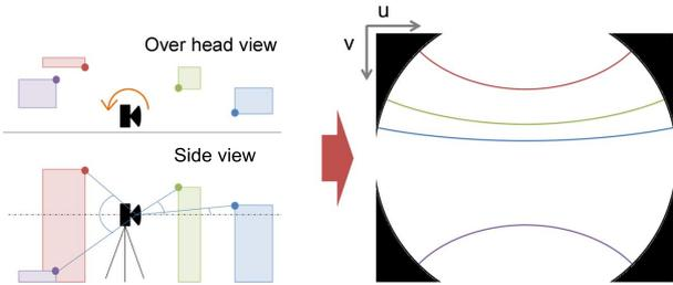
Fig. 1 Making feature point trajectories
