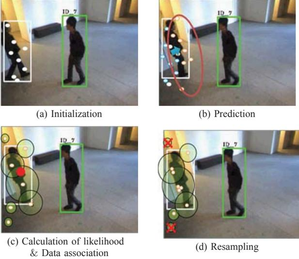
Fig. 4. Flow of particle filter
