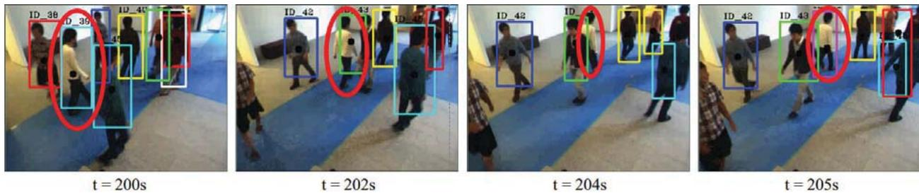
Fig. 8. Failure of human tracking
