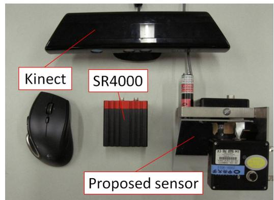
Fig. 20: Proposed sensor and other representative range image sensors
