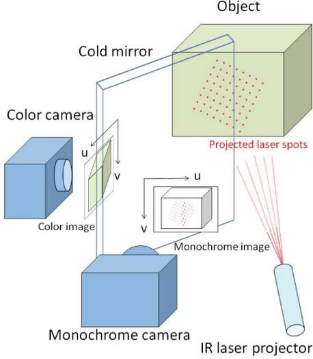
Fig. 1: Structure of the coaxial textured range image sensor
