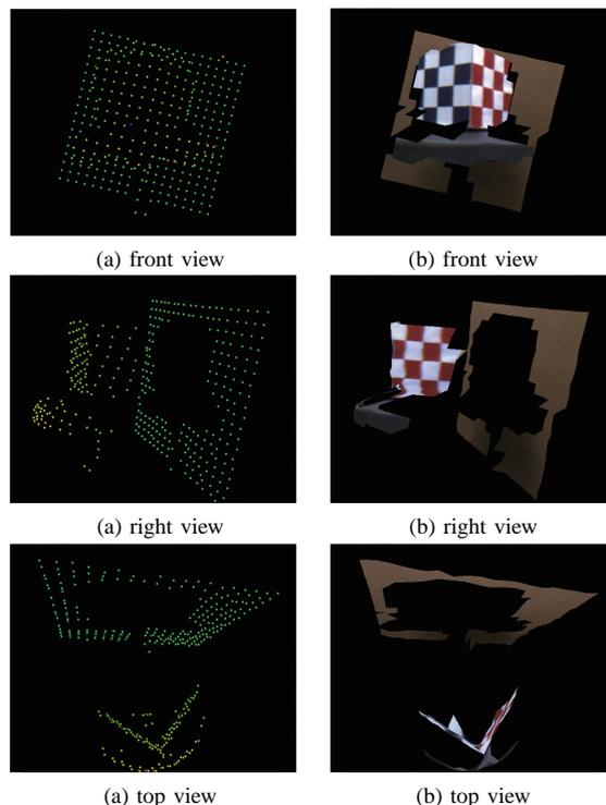
Fig. 12: Measurement results for Fig.8 (left: range image only, right: range image with color texture)
