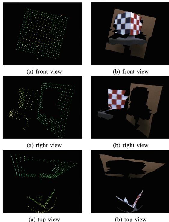
Fig. 12: Measurement results for Fig.8 (left: range image only, right: range image with color texture)
