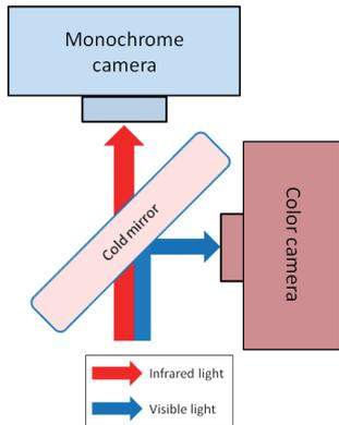
Fig. 4: Arrangement of the sensor
