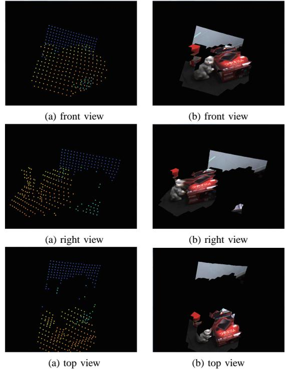
Fig. 14: Measurement results for Fig.9 (left: range image only, right: range image with color texture)
