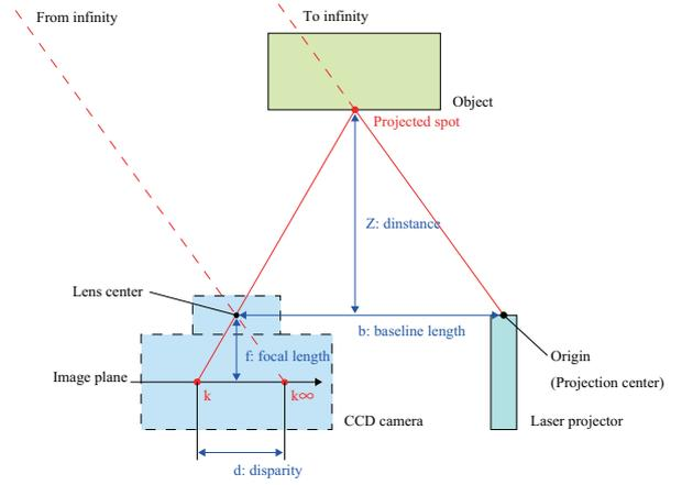
Fig. 2: Range image measurement
