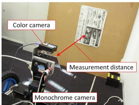
Fig. 16: Experimental setup to verify image disparities
