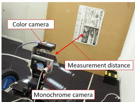
Fig. 16: Experimental setup to verify image disparities
