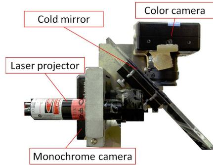
Fig. 6: Constructed sensor
