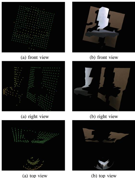
Fig. 11: Measurement results for Fig.7 (left: range image only, right: range image with color texture)
