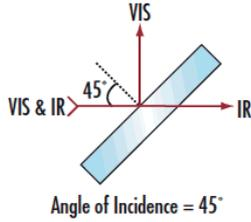
Fig. 3: Characteristics of the cold mirror [14]
