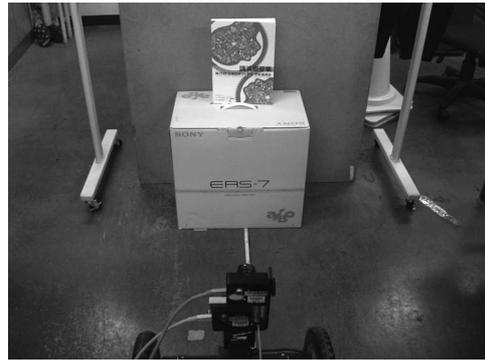
**Fig. 13** Measured object to evaluate measurement range
