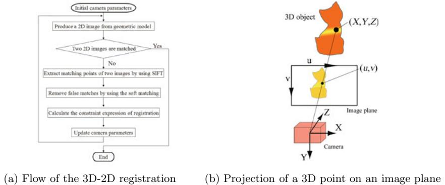
**Fig. 2.** Flow of the 3D-2D registration and projection of a 3D point on an image plane
