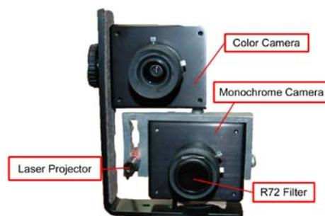
Fig. 1 Textured range image sensing system
