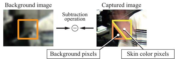
**Fig. 9.** Background subtraction at the pixel level.
