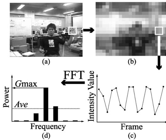
Fig. 4. Detection of hand waving using FFT.
