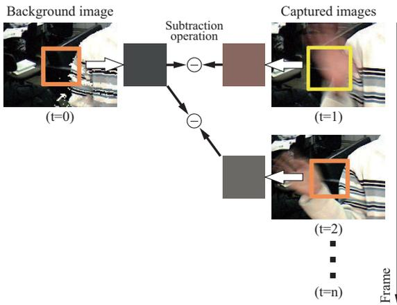
**Fig. 8.** Background subtraction in the region of the waving hand.
