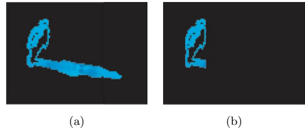
Fig.3 Removal of shadows ((a) Moving region in the sun (b) Moving region after the method to remove shadow is applied)
