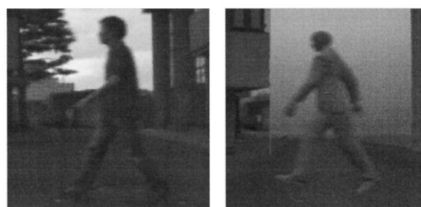
(c) Real image (F=16) (d) Output image by the camera simulator (F=16)
