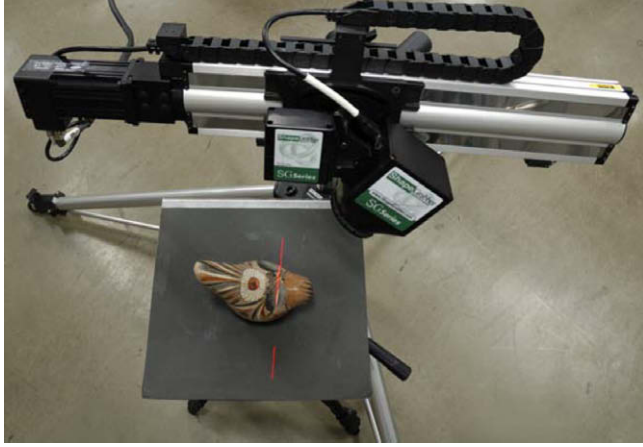
Fig. 8. ShapeGrabber range sensor with a target object.
