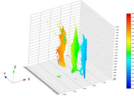
Figure 3. Point cloud; The blue points mean close to the camera, and the red ones mean far from the camera.
